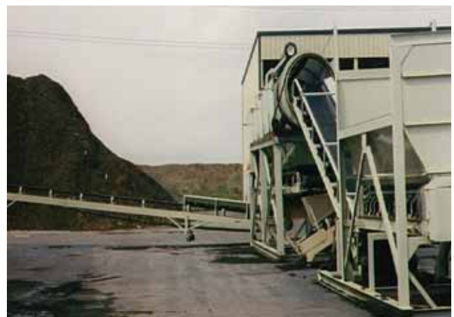
Figure 5b. Municipal composter, a form of in-vessel composting, combines processes from the turned pile and from the static pile techniques. It overcomes disadvantages and uses good points of each method.
